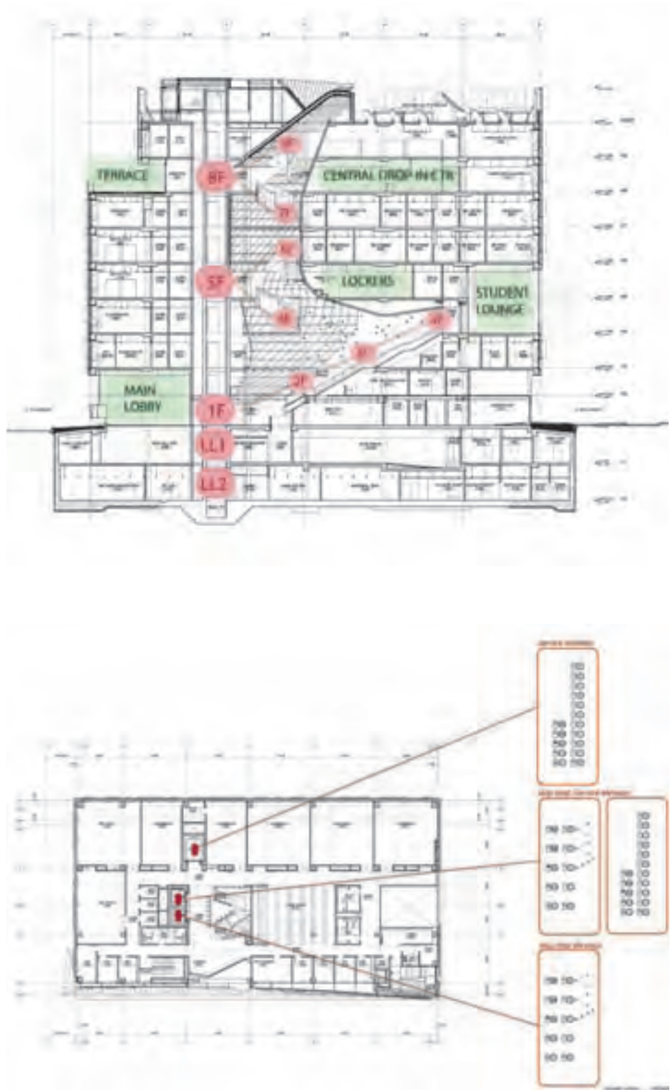
Diagram of the skip-stop elevator system
